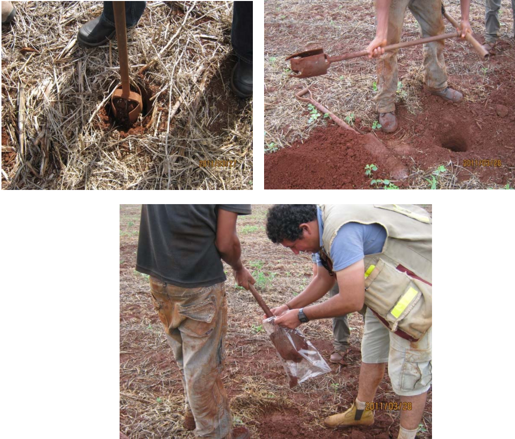
FIGURE 9-1: HAND AUGER DRILL FOR SHALLOW SAMPLES PARANÁ PROJECT (SOURCE: CIC, 2011)
