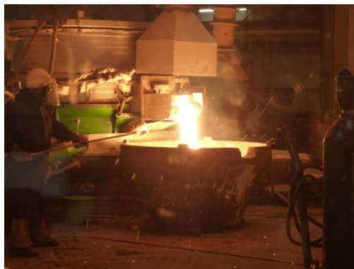
FIGURE 13-12: SLAG TAP FROM PILOT PLANT FURNACE (SOURCE: MAG, 2012)
