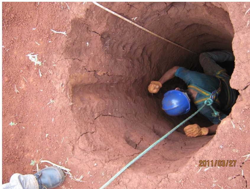
FIGURE 11-1: TYPICAL DEEP PIT SAMPLING Collecting Due Diligence Samples (Source: CIC, 2011)
