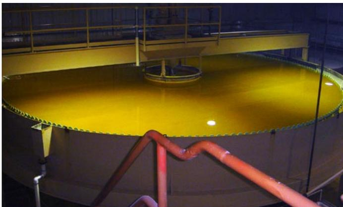
*The suspension of uranyl peroxide crystals is pumped to a cone-bottom thickener where the solids settle and concentrate. The liquid overflows the thickener and is routed to a Reverse Osmosis (R.O.) unit*
