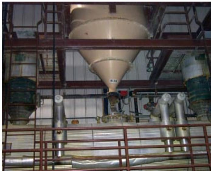
*Washed yellowcake is pumped to one of two rotary vacuum dryers. The slurry is dried under vacuums of up to 20 in. Hg for about 17 hours. The vacuum drier prevents the formation of insoluble uranium compounds in the final yellowcake product.*
